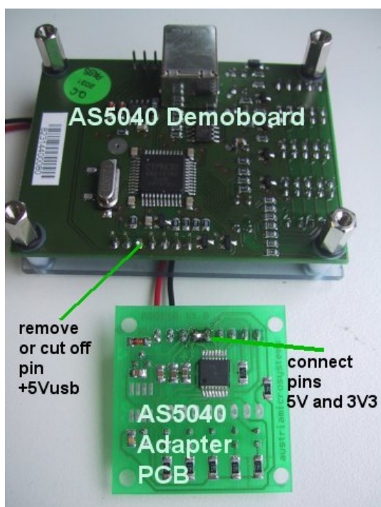
Figure 9: configuring the Adapter PCB for 3.3V operation
